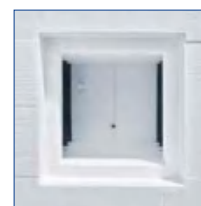
Inner Chamber of Exposed Heating Elements-type
